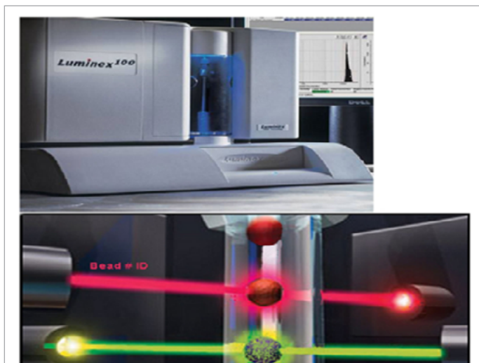
Figure 9: the top panel shows the luminex instrument. The bottom panel shows two lasers in the luminex instrument. One red laser identifies bead with attached HLA molecule and second green identifies the HLA antibody.
